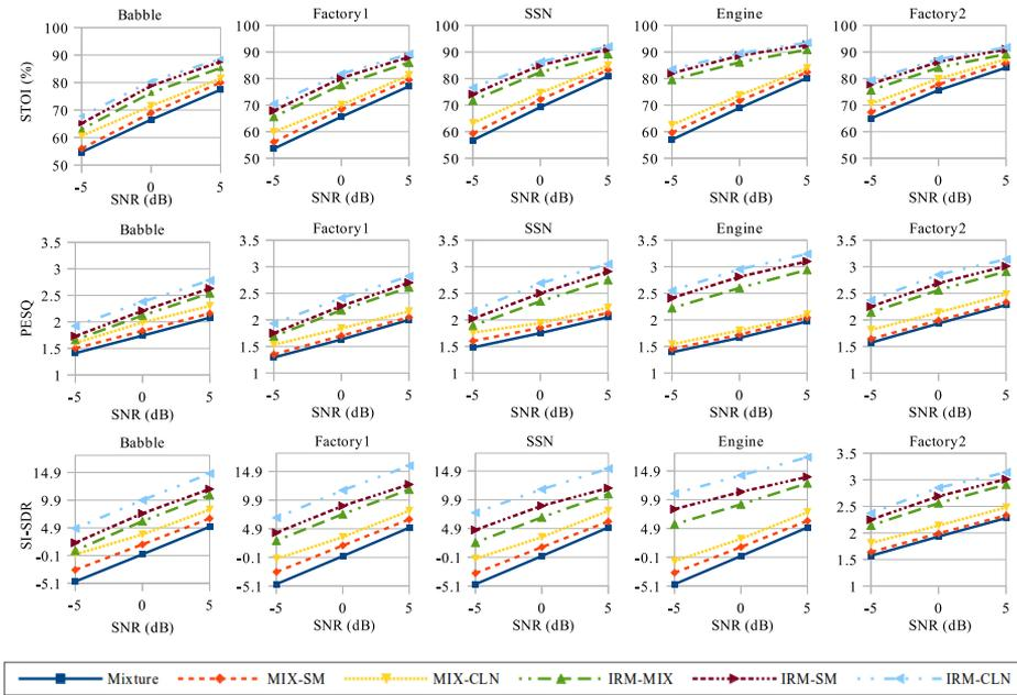
Fig. 6. STOI, PESQ, and SI-SDR comparisons between learned phase, noisy phase, and clean phase.
