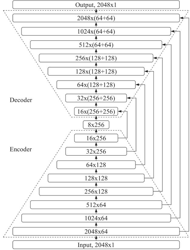
Fig. 2. A schematic diagram illustrating the architecture of the proposed model. The numbers represent the output dimension after each layer where  $M \times N$  denotes a signal with dimension  $M$  and number of channels equal to  $N$ . Note that the number of channels in the decoder is double of that in the encoder because of the concatenation of the incoming connection from the symmetric layer of the encoder. Arrows denote skip connections.
