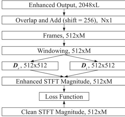
Fig. 1. Block diagram showing the steps involved in computing a frequency domain loss from the time domain frames at the output of network.  $L$  denotes the number of frames of size 2048, and  $N$  the length of the enhanced utterance obtained after overlap-and-add.  $M$  is the number of frames of size 512.  $D_r$  and  $D_i$  represent the real and the imaginary part of the DFT matrix, respectively.
