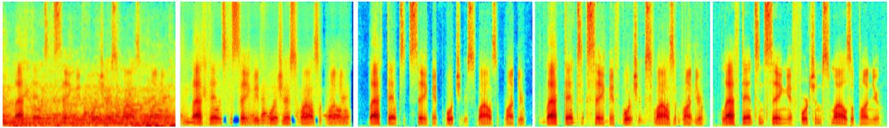
Figure 2: From left to right: noisy spectrogram (babble noise at -5 dB SNR); spectrogram of the signal enhanced with DNN; spectrogram of the signal enhanced with AECNN-T; spectrogram of the signal enhanced with AECNN-SM; clean spectrogram
