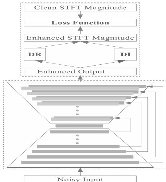
Figure 1: Schematic diagram of the proposed learning framework. Lower part is the network in the time domain and upper part shows the operations to compute the loss function in the frequency domain.
